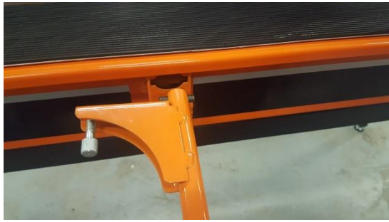
Insert both pinned shafts
